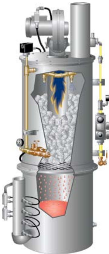
Cutaway view of the Armstrong International Flo-Direct water heater. The key to its efficiency is nearly complete utilization of combustion heat energy.
