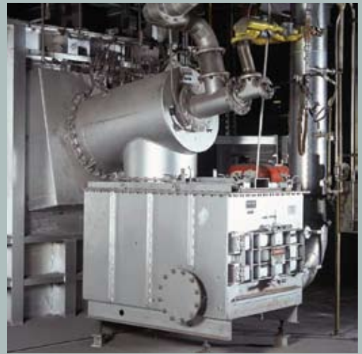
Bloom regenerative burners on an aluminum melting furnace improve efficiency by capturing heat that would otherwise be lost to the burner exhaust. Photo courtesy Bloom Engineering.
