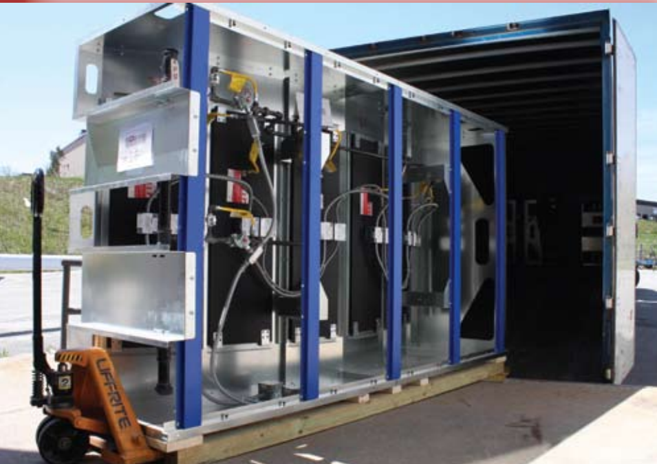
This compact module by Vulcan Catalytic permits rapid installation on an existing powder paint line, and can be used for pretreatment for a conventional convection oven, or for an all-infrared operation. Photo courtesy Vulcan Catalytic.
